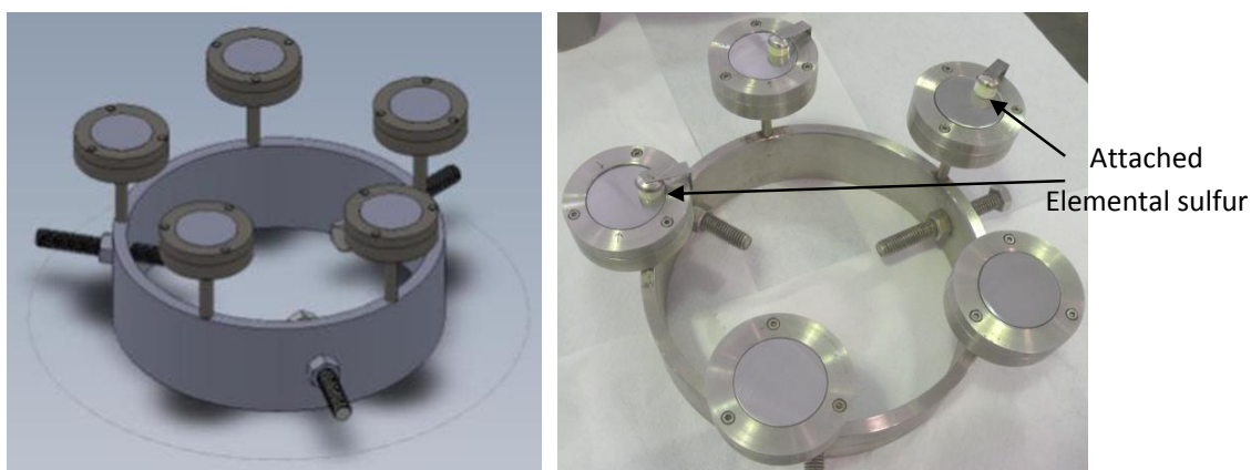
Figure 3: a) Sample holder setup for bottom of the line b) Elemental sulfur in contact with the steel surface
